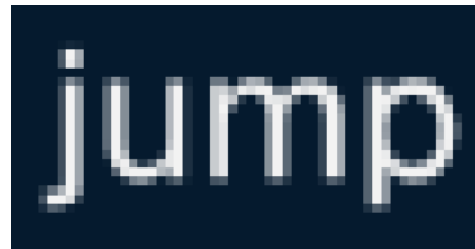
Figure 8: Without hinting, features like stems cannot be aligned on pixel grid boundaries
